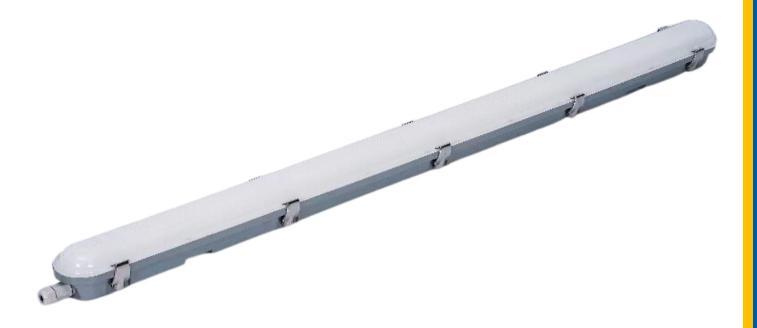
The Tezla Corrosion proof range are a high quality IP65 range with options from 600mm to 1500mm. Each size is available in a single or twin option and the fittings are all dual power as standard, meaning you can reduce the power to save energy if required. These fittings are highly efficient, with a lumen output of 130lm/W and are easily installed. The wide voltage driver means these fittings can also be used on sites with a 110V supply.
