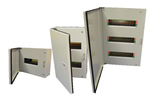
The Plymouth Metal Distribution Boards are surface mounted metal boards with a side opening door. All are supplied with din rail and neutral & earth bars. All boards are supplied with standard lock but this can be replaced for a lockable lock which uses a key
