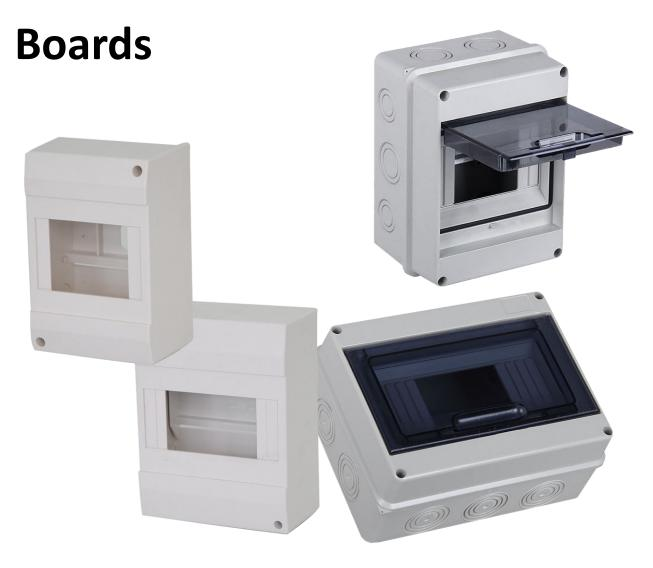
The Plymouth PVC Distribution Boards are surface mounted PVC boards, available with or without a vertical opening door. The are available in IP40 without door or in IP65 with the door. The boards are supplied with all accessories necessary for your connections such and din rail and earth bars. All come with knockouts for easy install
